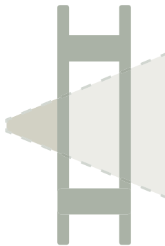
Wood, plaster walls loss: 5 to 20%
